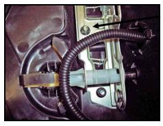
Step 5: Remove Nut, Hit Bolt with Hammer until flush with metal bracket. Won't take much effort. Now turn seat right side up.
