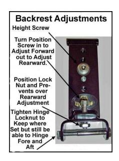
A driver's backrest that becomes part of your seat. No bars in the way of the driver's hips and legs or passenger's legs. Folds forward to ease passenger getting on or off and adds to safety by getting out of the way in sudden stops. Includes up and down height adjustments, as well as driver seating position, back and forth, to help driver sit upright to avoid slouching, a big factor in driver fatigue.
