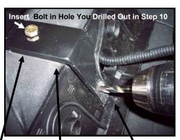
Step 12: Place Bar as shown. Install furnished Hex Head Bolt and Nut snuggly, not tight yet. With 9/32 Bit place through Hole in Bar and Drill through Plastic. Install furnished Flathead Bolt, Washer and Nut and Tighten. Then tighten Nut on Hex Head Bolt.
