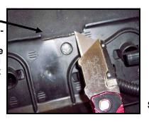
Step 10: Drill out Bolt Hole to 9/32".
