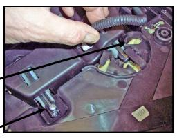
Step 4: Pull Strap and Slide Butt Pad forward. Remove Plastic Cover.
