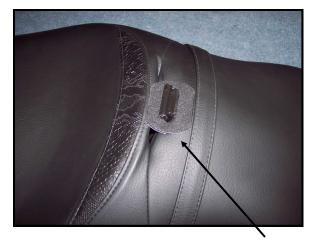
Step 6: Install the peel and stick boot included with your new backrest, over the tube now above seat. This will protect your seat cover from backrest hinge action. Will stick on rear only, front seat will move under boot.
