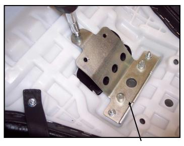
Step 2: Turn seat over, remove bracket covering slit in seat.
