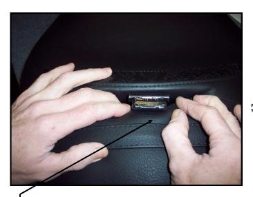
Step 4: Slide bracket up threw slit in seat and bolt stock bracket back in place in reverse of step 2.
