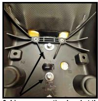
Step 6: Line up mounting bracket threaded holes up with holes you drilled. Insert bolts through washers (cut washer front hole) and screw into the threaded holes in mounting bracket and tighten.
