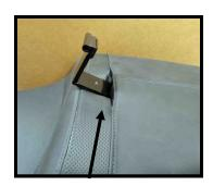
Step 5: Slide mounting bracket into slit, working it under seat foam resting on top of seat base inside seat.
