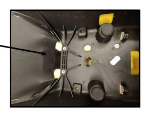
Step 3: Measure back from front edge and center mark for holes.
