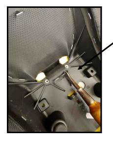
Step 2: Remove staples on fly, tuck out of the way back in seat, to allow our mounting bar to slide on top of seat base.
