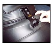
Step 10: Install bar attached to pad to tube now sticking out of seat. Slide in bolt furnished and tighten bolts. Make tight enough that backrest will stay in place, but will still hinge back and forth.
