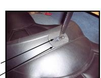
Step 1 Lay hole end of T-Bar flush against seat base to
