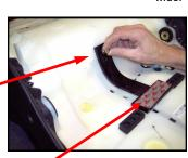
**Step 9** Tuck all wiring in area, down between cross frame and black wiring junction box, to assure no wire gets pinched.
