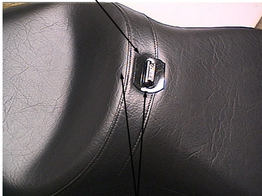
Step 3) Measure 1 1/2" back from top of rise to make slit. Center side to side.
