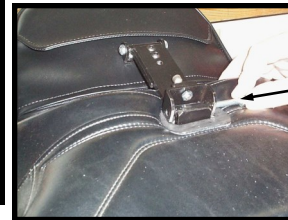
Step 8: Install bar attached to pad to tube now sticking out of seat. Slide in bolt furnished and tighten bolts. Make tight enough that backrest will stay in place, but will still hinge back and forth.
