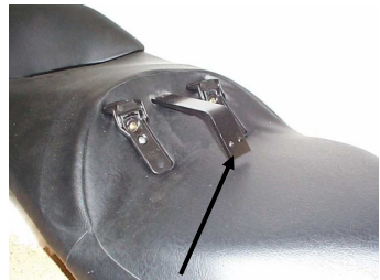
Support Bar Shown slid into Seat without Adjustable Pad Installed, related to Step 11 and 12.
