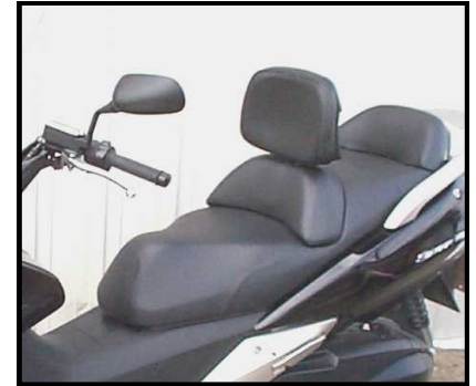
Step 14: Finally, attach Utopia Driver Backrest to Tube now sticking out of Seat. Install 2 1/4" Bolt and Crimp Nut Furnished through Bar on Backrest and Tube and Tighten Nut. Follow Backrest Adjustment Instructions on Front Page of this Installation Instructions.
