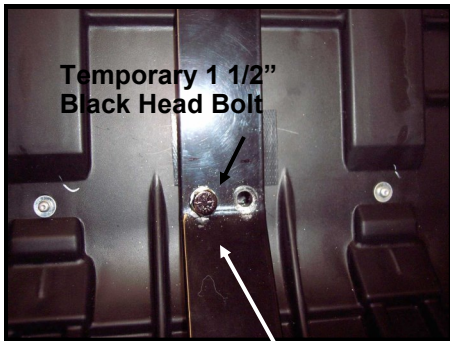
Step 13: Temporarily Install 1 1/2" Bolt with Black Head, though Anti-Flex Bar, Seat Base and into Threaded Holes in Support Bar that You Installed on back of Stock Adjustable Pad. Draw up enough to Install one of the 1 1/4" Bolts with Lock Washer in the Other Hole. Now Remove Black Head Bolt and Install the Other 1 1/4" Bolt and Lock Washer. Discard 1 1/2" Bolt.
