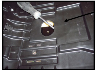
Step 11: Install the Two 1" Bolts with Lock Washers, through Support Bar, Seat Base and Into Threaded Holes on Inside Bar You Just Inserted into Stock Adjustable Pad and Tighten with Socket or Wrench that fits in area of Bolts.
