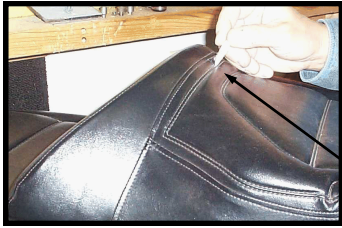
Step 3: Measure from rear of seat forward 8 1/2". Feel for and measure foam, not loose seat cover. Mark and center side to side. (see Step 3 below).
