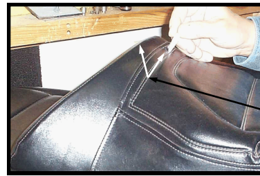
Step 5: With a long serrated knife cut hole through Boot and Cover 1 1/2" wide into foam, clearing foam from area where you just drilled in step 2. Boot will keep you from cutting too wide.
