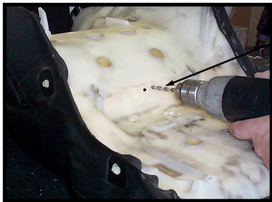
Step 2: Drill 9/32" Holes in Seat Base
