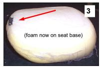
3. Slide foam over installed bar, as shown in picture 3. Tube should be close to level with the surface of foam.
