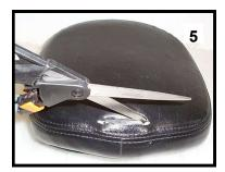
5. Carefully make a slit to allow it to come through the now installed cover, as shown in picture 5. "DO NOT CUT ANY THREADS WHERE COVER IS SEWN TOGETHER." Cut no wider than necessary.
