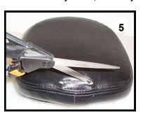
5. Carefully make a slit to allow it to come through the now installed cover, as shown in picture 5. "DO NOT CUT ANY THREADS WHERE COVER IS SEWN TOGETHER." Cut no wider than necessary.
