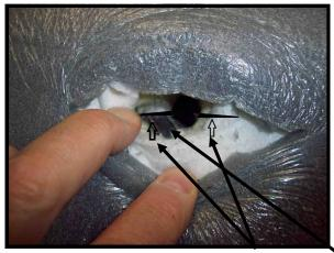
Step 7: Cut slit with long serrated knife, through top of seat foam through bottom of foam, 1" on each side of hole in seat foam and move black wire into slit you cut, on left side of hole. Careful not to cut wire.
