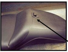
Step 9: Turn seat upright. Lay mounting bracket in place, lining front hole with hole you just drilled in seat base. Loosely install bolt with 1' and 2" washers. Center rear hole in bracket on seat base, mark and drill. Install bolt and washer and tighten both bolts, making sure all is centered.
