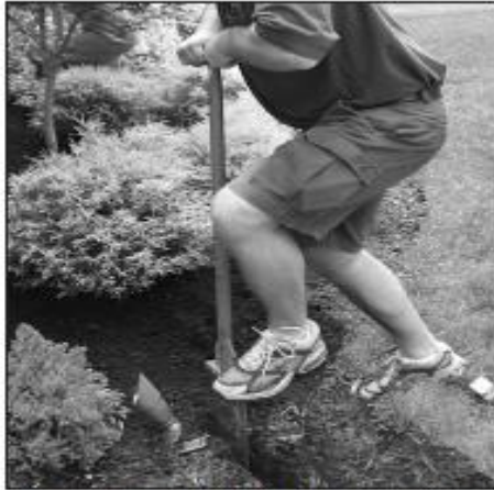
The CAST Trenching Tool (CWTT) cuts a narrow 8" deep trench ideal for laying wire.
