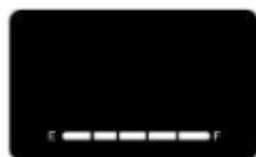
When the battery displays fully lit, it is fully charged. E flashing indicates battery low, It can be used after recharged. Don't use the product when charging
