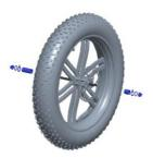
(2) Place the front wheel in the front fork card slot and lock it with a 15mm wrench.
