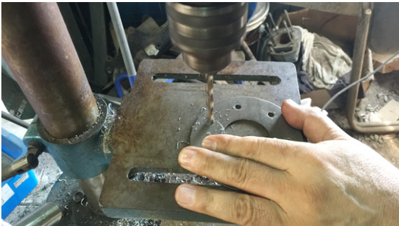
06 Open the rivet holes in the cover plate with a 6mm drill bit.
