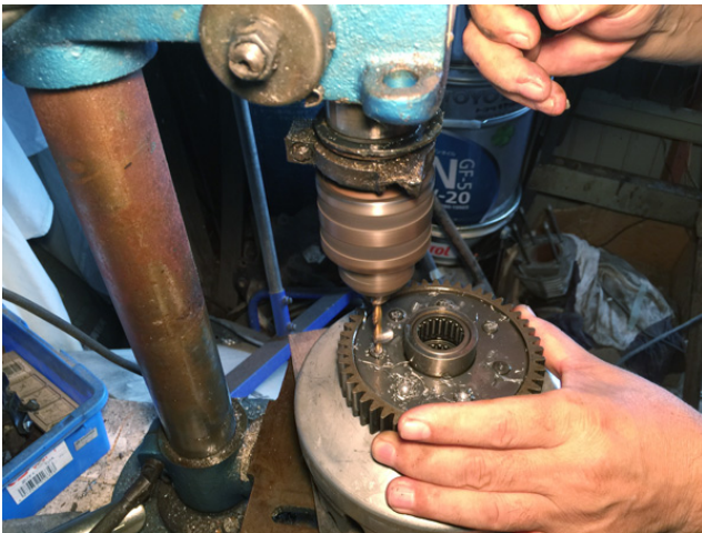
01 Start by separating the outer clutch from the rest of the clutch components.
