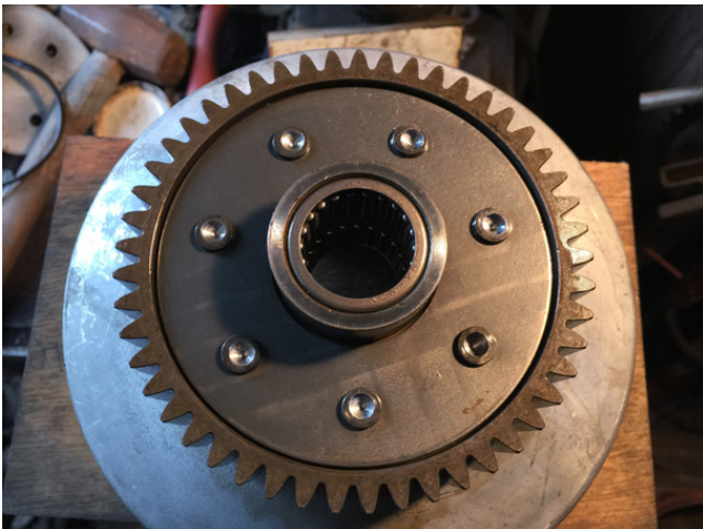
02 Mark the center of each rivet with a punch and using a 5mm drill bit, drill out the rivet head to a depth of 3-4mm.
