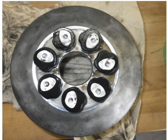
03 Use a chisel to strike the rivet heads to remove them and then remove the cover plate.
