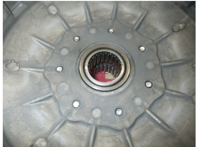
09 For extra security you can use a punch topeen the bolts to the outer clutch basket.
