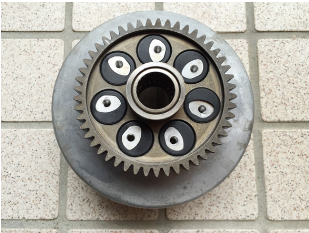
07 Insert the new clutch rubbers and reassemble the outer clutch.
