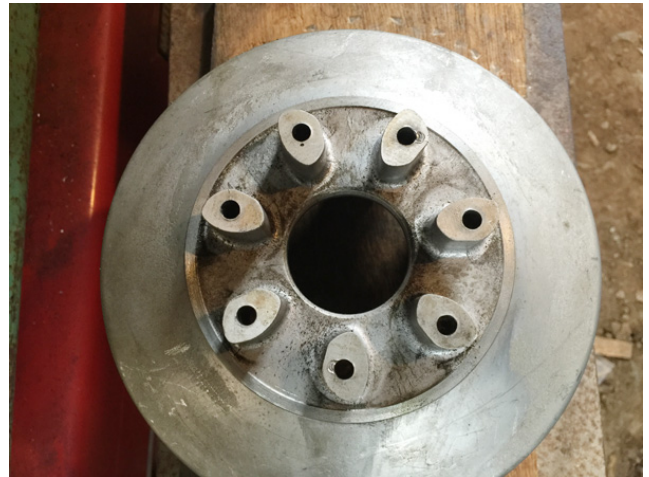
04 Remove the ring gear and the old dampers and using a 4mm punch, drive or press out the rivets from the outer clutch.
