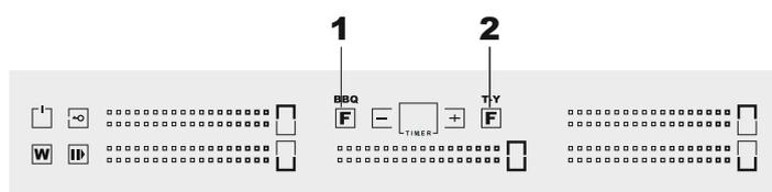
To activate the **Barbecue** mode, press and hold the function key **F, 1** for approx. 5 seconds. The indicator will illuminate and the displays will show **b** and **q**. The heating level will be automatically adjusted.
