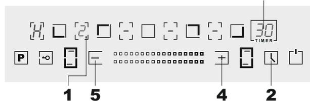
The timer can be set for multiple fields simultaneously. At the same time, the display will show the smallest of the set times. Decimal point **1** of this field is flashing. In other fields that have activated timer function, signal points are lit and not blinking.
