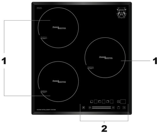
**Economy:** energy consumption is several times less than that of any other hobs. Touch sensors are made fit the diameter of the zone of generation of vortex flow by the size of the bottom of an utensil, if it lies within acceptable limits.
