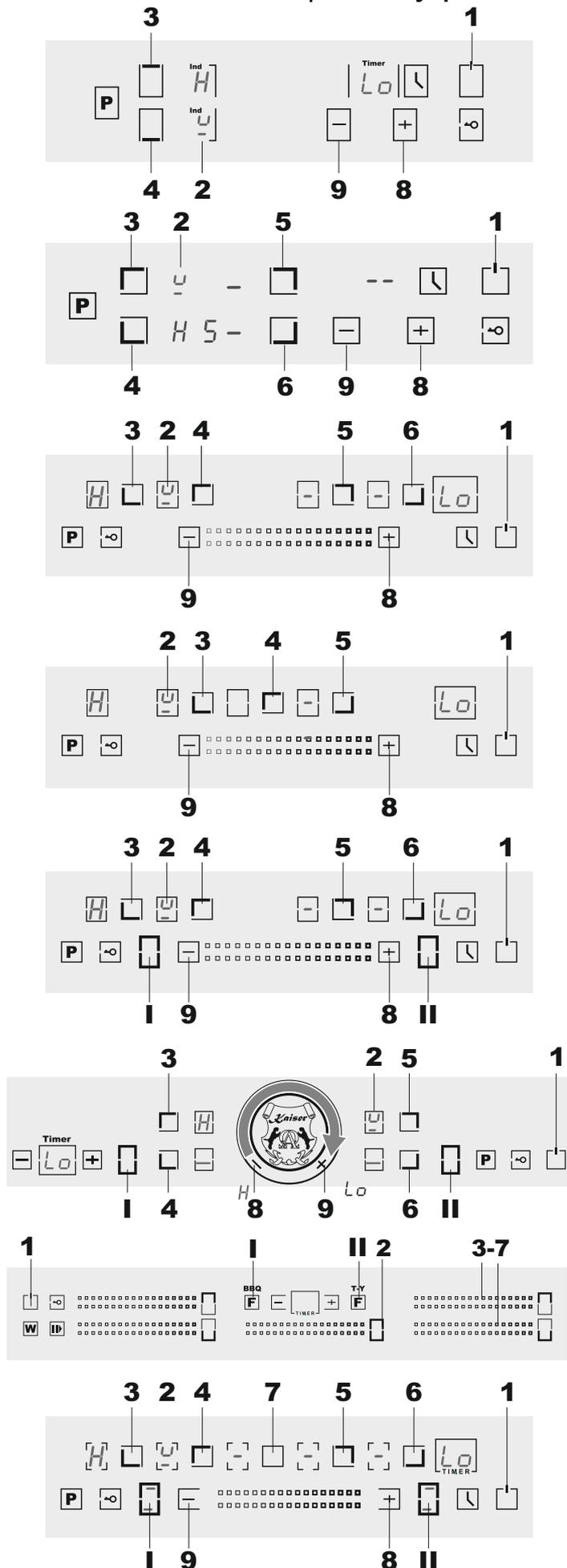
The **ON/ OFF** key **1** has always priority in the switch-OFF function.
