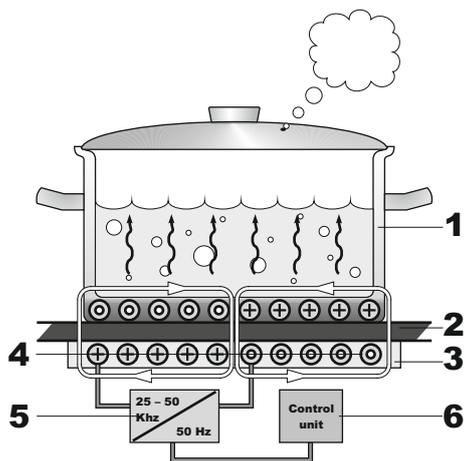
1. Utensil made of ferromagnetic material
