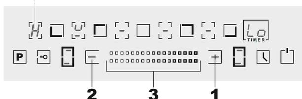
For more comfortable selecting of the power level for models with slider control you can set the power level from **0** to **9** by touching the required position on the control panel.
