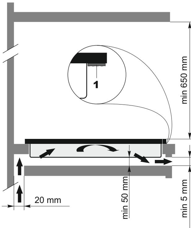
The cooking hob should be fitted into the counter top as illustrated on the figure. Apply the supplied seal **1** over the whole perimeter of the hob if it has not been preinstalled.
