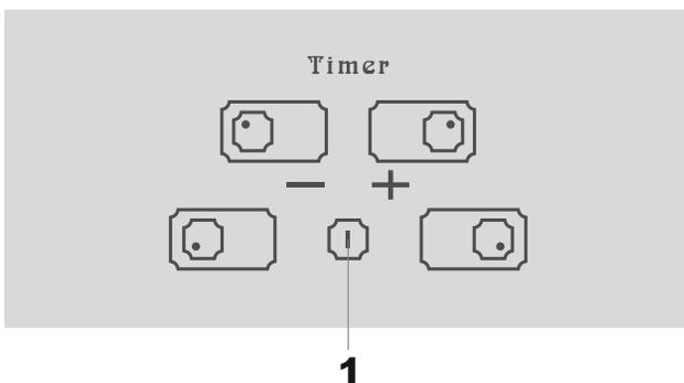
Be especially careful to keep the sensor keys clean since soiling could be mistaken for finger contact by the appliance. Never put anything (pans, tea towels etc.) onto the sensor keys! If food boils over onto the sensor keys, we advise you to activate the **OFF** key **1**.
