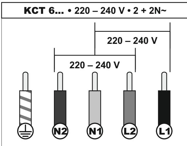
If the appliance is to be connected directly to mains terminals, fit a switch with minimum aperture of 3 mm between the contacts. Make sure that the switch is of sufficient capacity for the power specified on the appliance's data plate, and compliant with applicable regulations. The switch must not break the green-yellow earth wire. The socket or switch must be easily reachable with the cooking hob fully installed.
