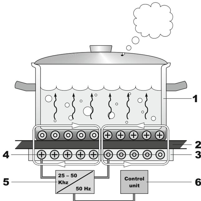
1. Utensil made of ferromagnetic material
