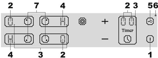
After a reset all displays and LEDs glow for approx. 10 seconds. When this time is over all displays and LEDs extinguish and the control is in the **stand-by mode**.
