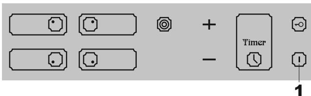
Immediately switch off the cooking zone after using with the respective sensor key **ON/ OFF, 1** and not just by pan recognition.
