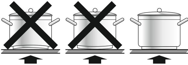
When one makes use of heating elements, we advise receptacles with flat bottom having same diameter or lightly higher than that of the hot area.
