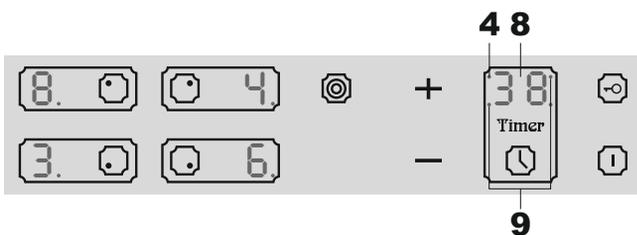
It come sound signals. The decimal point **4** of the relative heating zone illuminates. It informs that timer has been activated. The timer function will start up automatically for the selected heating zone only.
