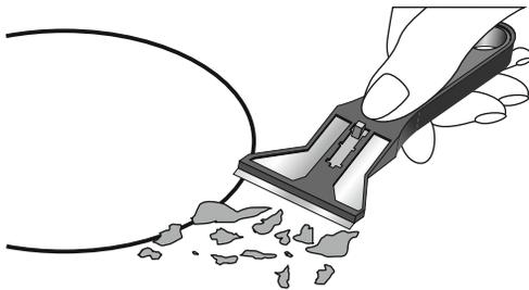
Pieces of aluminum foil and plastic material which have inadvertently melted or sugar remains or highly sacchariferous food have to be removed immediately from the hot cooking area with the special scraper. -This is to avoid any possible damage to the surface of the top.
