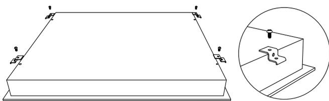
The cooking hob should be fitted into the counter top as illustrated on the figure. Apply the supplied seal **1** over the whole perimeter of the hob if it has not been preinstalled.
