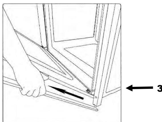
The track system is easily to be removed to clean the oven. The construction is made of stainless steel, which excludes the possibility of corrosion formation.
