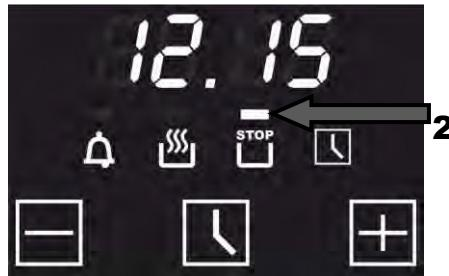
The display shows the countdown time, symbol **2** appears on the display to confirm the successful setting and the current time appears again.
