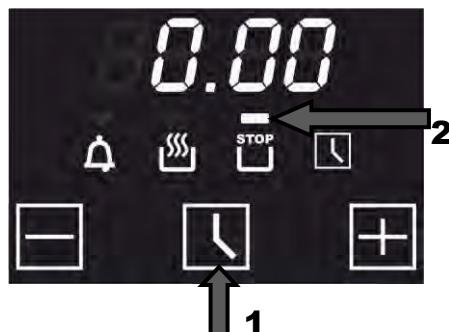
Before setting the end of cooking time you have to set the **oven operating function grill** and the **temperature** (see chapter “Electric grill”).
