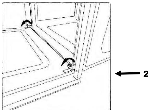
The tracks of every griddle resist a loading up to 15 kg in the completely pulled out state.
