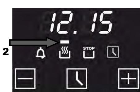
After the end of the countdown the oven emits the triple sound signals with the interval of 2 seconds during two minutes to inform you that all processes in the oven are switched off. The symbol **2** will continue to flash after the end of emitting the sound signals.
