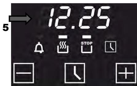
In our example the oven should be turned on at **12:25** (5) with the functions “Grill + Thermocirculation” and be turned off at **12:55** according to your setting.
