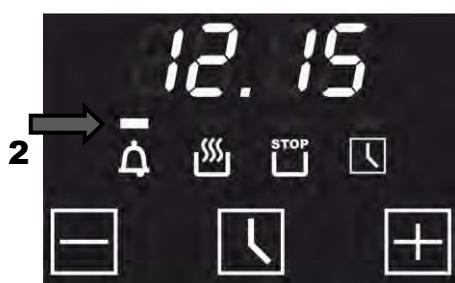
After a few seconds the timer starts the countdown, the display shows the countdown time, the symbol **countdown timer 2** appears. By pressing the button **1** you can call up the current time indication for 5 seconds.
