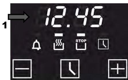
The end time (1) appears on the display, that accords to the current day time plus duration (in our example **12:45**, that means plus 30 minutes).
