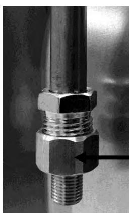
On the pipe **1** is a nut **2**, with a fixed service-adapter **3**, which is for gas service personal only. The gas connection with this adapter is prohibited. Before connecting the gas the service-adapter **3** has to be removed.
