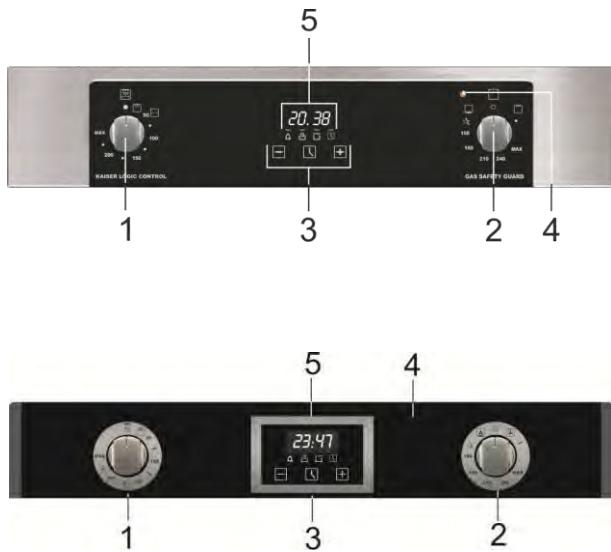
1. Rotating knob for grill temperature control, for turning on the turnspit and oven inner light
