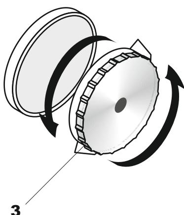
Filters with a charcoal can absorb odours until they are saturated. They cannot be washed or regenerated and should be replaced at least every 6 months or more frequently in case of very intensive use.
