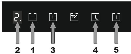
The backlight of button is on, the cooker hood's fan speed goes lower. The display **2** shows the fan speed.
