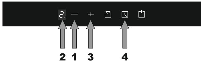
The backlight of button is on, the cooker hood's fan speed goes lower. The display **2** shows the fan speed.
