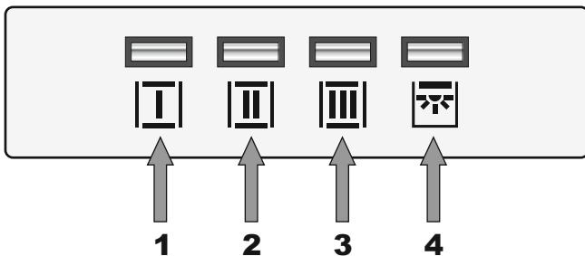
The button **4** is used to turn on and off the extraction hood lighting; independently of the engine work status, push this button to switch on/ off the lighting. The indicating light **8** turns on/ off accordingly.
