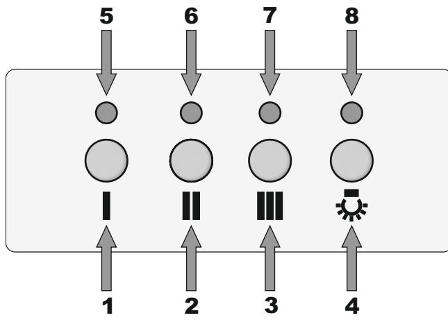
According European Norms 65/2014 and 66/2014 the hood with motor power more than 260W may work on high speed **III** only 7 minutes, after 7 minutes the speed is changed to medium speed **II** automatically.
