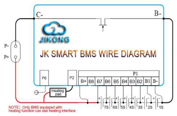
figure.5. wiring mode of 7-string battery pack system
