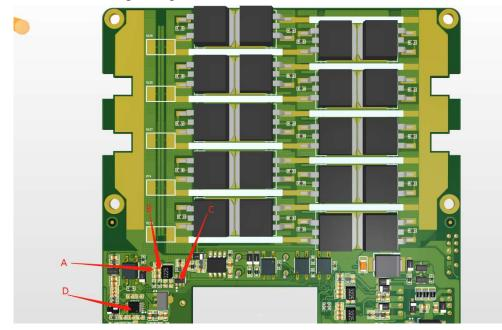
**Step 2:**After power on, test the voltage between A and B points in the diagram. If the voltage is between 4.5~5.2V, it is necessary to replace chip D, which is MDT10F272. After switching off and replacing the chip, turn on the machine again to test whether the functional fault is eliminated.
