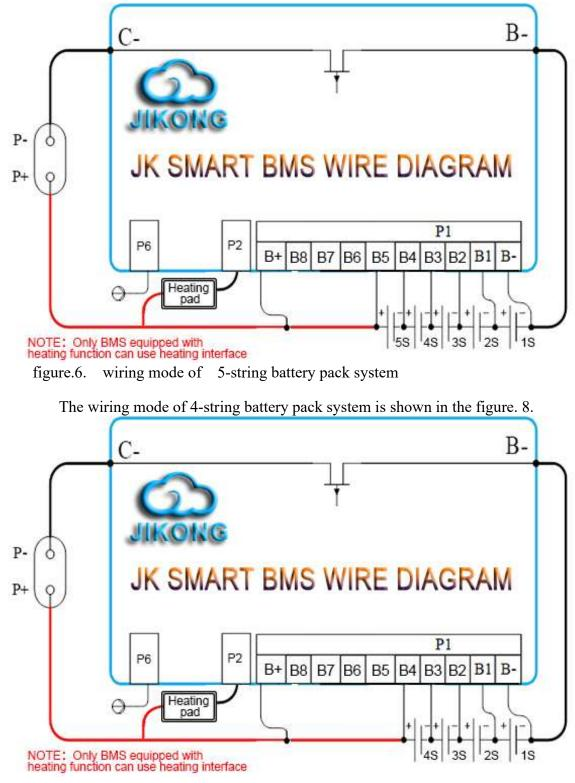
figure.8. wiring mode of 4-string battery pack system
