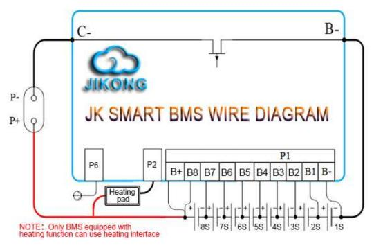
Figure 4. wiring mode of 8-string battery pack system The wiring mode of 7-string battery pack system is shown in the figure.5
