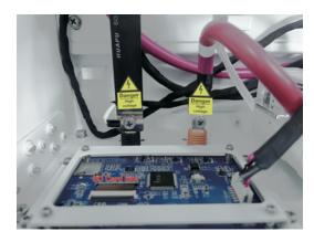
Note: When inserting the SD card, unplug the battery power cord and manually turn the air switch to the off position.
