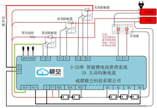
Wiring mode of serial battery pack system
