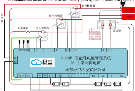
The connection mode of the 16 series battery pack system is shown in Figure 6.
