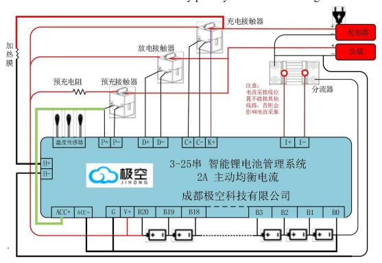
The 20 Strial battry wiring diagram is shown.
