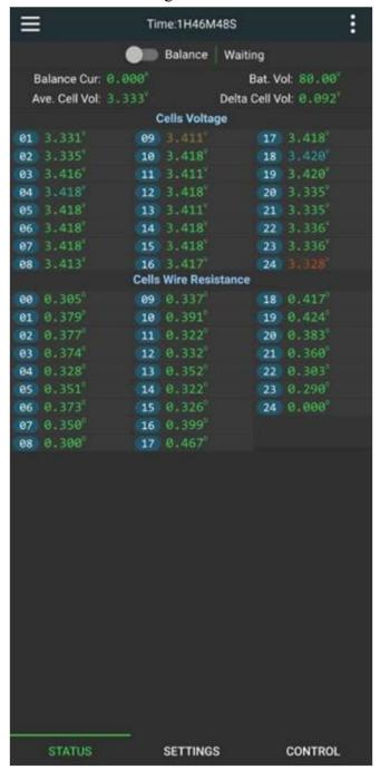
On the Real-Time Status page, you can view information such as switch status, charging current, discharge current, temperature display, protection alarm, individual voltage, total battery voltage, maximum pressure difference, average single voltage, balanced status, balanced current, balanced line resistance, etc.
