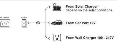
RECOMMEND TO DISCONNECT THE POWER STATION WHEN IT FULLY CHARGED. WHEN CANNOT CHARGE THE POWER STATION, PLEASE CHECK IF THE RESET BUTTON IS ON.
