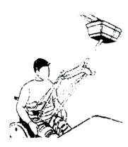
6b. When using a ceiling lift, the chair must be positioned at right angles to the track. (The sling is not suitable for use with all ceiling lifts. Please check with your supplier.)
