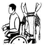
1. Take hold of the sling at base of back section ensuring that the quilted side will fit against the person's body. The handle loops at the back will then be visible when the sling is fitted.
