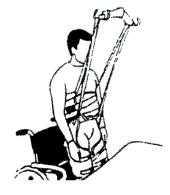
7. Raise the carry bar just enough to tension the straps and ensure that they are still securely attached. The person can now be raised to the standing position. To remove the sling, carry out the fitting procedure in reverse.
