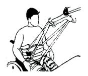
6a. Lower the carry car of the ceiling lift o approximately the seated person's eye level height. Attach all four straps to the carry bar using loops of the same color. Block the person's knees with a bed or frame. (Instructions also apply to fig. 6b.) The sling is not suitable with all ceiling lift. Please check with your supplier.
