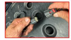
Install the inline harness between the tailgate side and truck side harnesses
