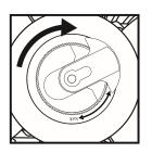
Step 5: Turn the fan grill and make sure the arrow sign aligns with the lock position.
