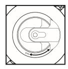
Step 2: Turn the fan grill until the arrow sign aligns with the unlock position.
