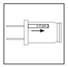
Close fuse cover. Slide closed the fuse access cover on top of attachment plug.
