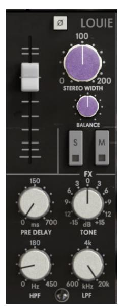
stereo width controls the balance between side and mid channels for any stereo microphone, 0 being all mid, 200 being all side, and 100 being its natural state and default position.
