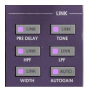
The **LINK** section allows you to synchronize knobs between all microphones, so that each microphone has the same pre-delay, tone, HPF, LPF, or width setting.
