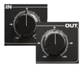
**INPUT** and **OUTPUT** control the gain of the signal before and after it hits the compression stage, respectively. Default is 0dB, range is -10dB to +10dB. Note: when auto gain is enabled, the output can be changed to offset the automatic gain control.
