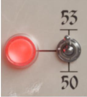
**53 / 50** switches between the two amps modeled in the plugin (see **Chapter 4** for more info). The light turns Red for 53 and Yellow for 50. Defaults to 53.
