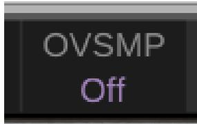
**OVSMP** sets the oversampling rate for DEATHWESTERN. Its default is Off, but it can go up to 16x. Oversampling increases CPU usage but can reduce aliasing.
