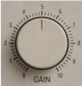
**GAIN** increases the signal gain into the first stage of the amp model, and acts like the preamp gain on the real thing. Goes from 0 to 10, defaults to 5.
