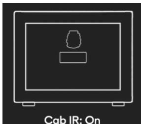
**Cab IR** toggles our speaker cabinet emulation, which uses the Impulse Response captured at The Panda Studios (see **Chapter 4** for more info). If you're using another IR or a real cab, disable this. Cab IR defaults to On.
