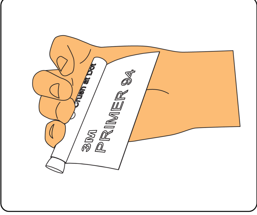
Step 3: Break primer ampoule by firmly pressing the black dot on the container, which will produce a popping sound. Keep squeezing the dot until liquid appears on the application pad at the end of the ampoule, and continue doing so until all the liquid has been used
