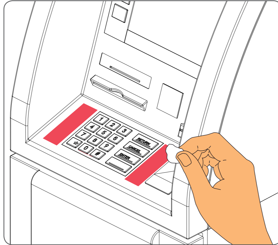
Step 2: Thoroughly clean the area shown using cleaning sachets provided. The area around the PIN Pad must be completely clean for the best adhesion. Allow to dry for 5 minutes.
