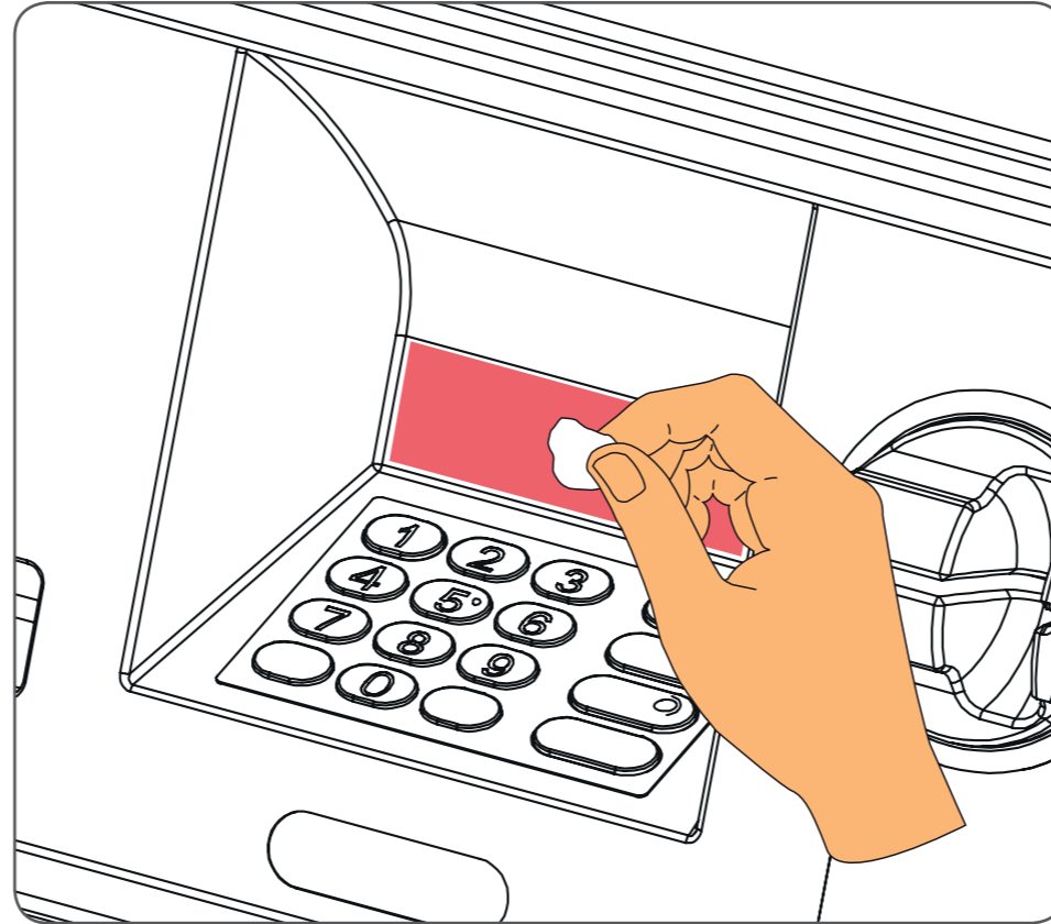
Step 2: Thoroughly clean the red area shown using cleaning sachets provided. The area around the PIN Pad must be completely clean for the best adhesion. Allow to dry for 5 minutes.
