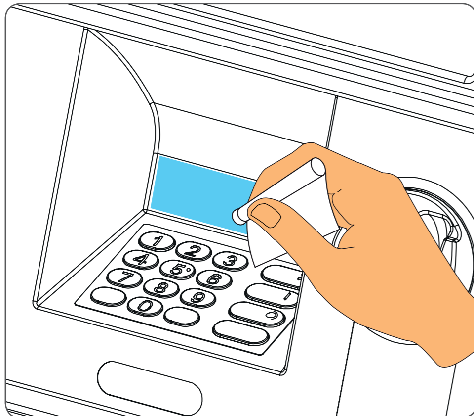
Step 4: Brush the primer onto the area shown. Ensure complete coverage of PINGuard® footprint area. Allow to dry for 5 minutes.
