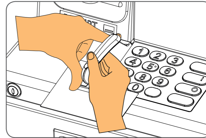
Step 7: Place the PINGuard® onto the ATM as shown. Once correctly aligned apply heavy pressure to the base for at least 2 minutes! This will remove any air bubbles and is vital for good adhesion. Leave for 5 minutes for bond to cure.
