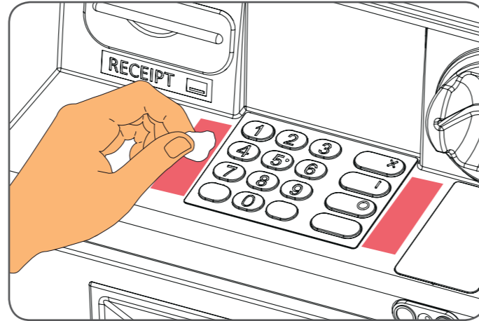
Step 2: Thoroughly clean the area shown using cleaning sachets provided. The area around the PIN Pad must be completely clean for the best adhesion. Allow to dry for 5 minutes.
