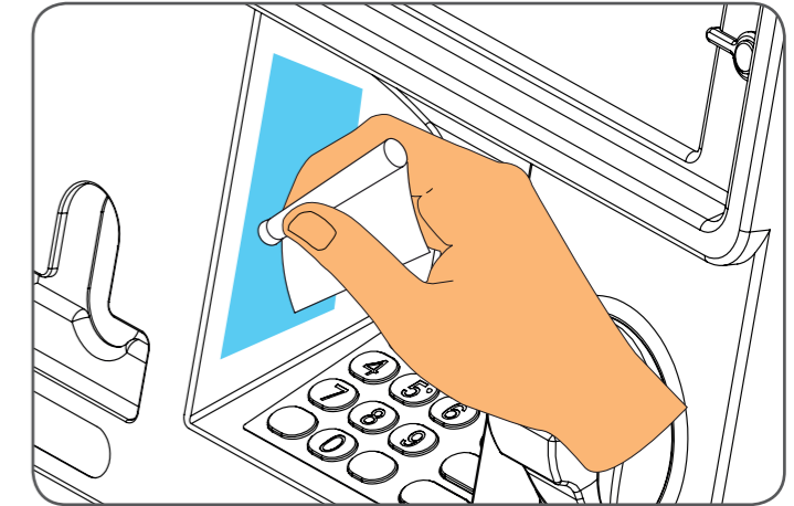
Step 4: Brush the primer onto the area shown. Ensure complete coverage of PINGuard® footprint area. Allow to dry for 5 minutes.
