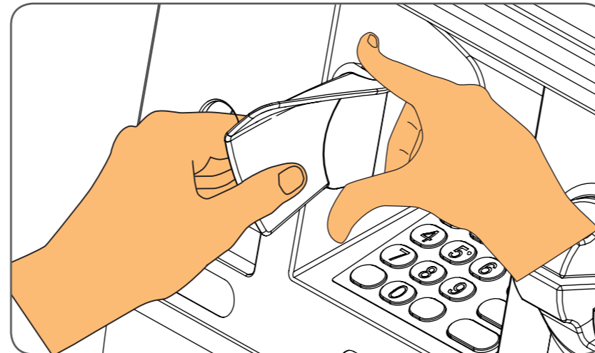
Step 6: Place the PINGuard® onto the ATM as shown. Once correctly aligned apply heavy pressure to the base for at least 2 minutes! This will remove any air bubbles and is vital for good adhesion. Leave for 5 minutes for bond to cure.
