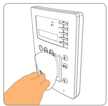
**Step 5:** Then carefully align the PINGuard® wings as before and gently press into position (if they are not in the correct position gently peel them off and reapply in the correct position).
