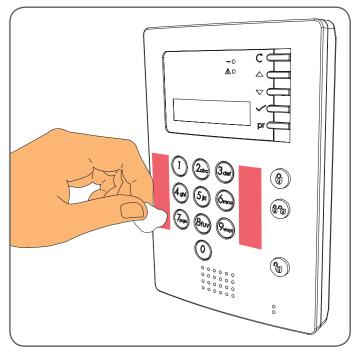
**Step 3:** Thoroughly clean the area shown using cleaning sachet provided. Ensure that it is absolutely clean. Allow to dry for 1 to 2 minutes.
