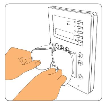
Step 1a: Take both the left and right PINGuard® wings and offer them up to the key pad as shown. Making sure they are in a good position to bond to the terminal. Ensure that the wings are positioned for the good access for the user.
