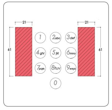
**Step 1b:**Alternatively you can check that the hatched area shown is clear and able to be take the adhesive of the PINGuard®.
