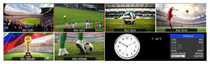
The lower right corner display of the menu and status information. The CH1, CH2 are the channel selection of the 2 audio sources for audio mixer. There is a real-time Digital clock/Analog clock displayed beside the menu.
