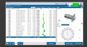
9x Dynamic Diameters 2x Arc Radii 4x Axial Distances 3x Groove Diameters 1x Cylindricity 1x Chamfer Angle MEASURING CYCLE TIME: 5.6 seconds!
