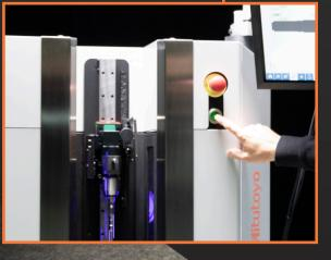
Roundtracer Flash is designed for ease of use: there is an open loading area with no obstructions and an ergonomic tailstock system for easy part clamping. The graphical user interface - via a touchscreen monitor - provides excellent ease of use.
