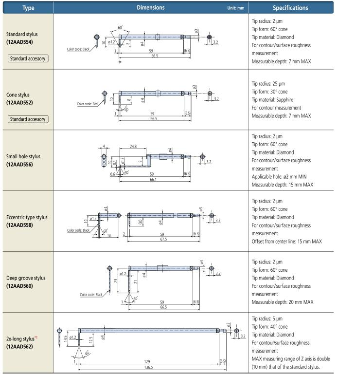
\*1: Measuring force is 4 mN and the Z-axis resolution is double that of the standard stylus.
