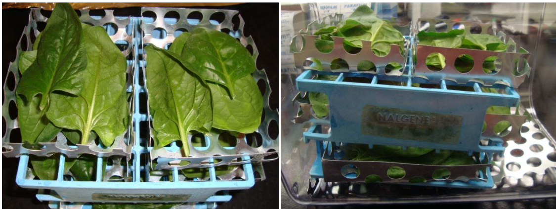
Figure 2.9. Six samples randomly positioned on an autoclaveable test tube rack (left); samples inside of the sample chamber which is located inside the treatment chamber (right).
