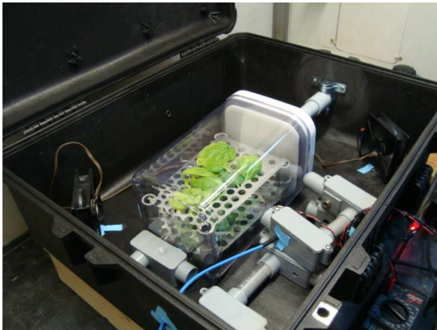
Figure 1.2. A smaller sealed sample chamber containing spinach samples inside the larger treatment chamber.
