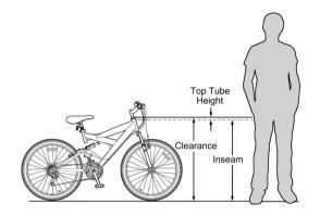
CAUTION: For safe and comfortable riding there should be a clearance of no less than 1 inch between the inseam area of the intended rider and the top tube of the bicycle frame, while the rider straddles the bicycle with both feet flat on the ground.
