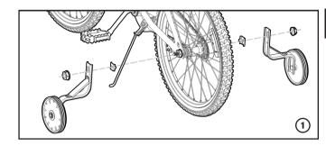
WARNING: The inner axle nut which holds the rear wheel on should not be removed or loosened while installing the training wheels. See Figure 1.)
