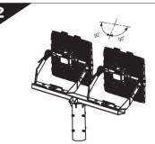
Adjust the orientation of the luminaire to achieve the desired lighting position and fasten the screws.
