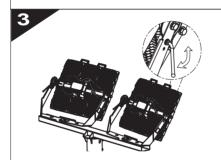
Loosen the handle of the luminaire's bracket.
