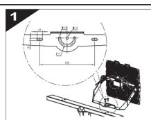
Fix the luminaire on the mounting bracket by screws.
