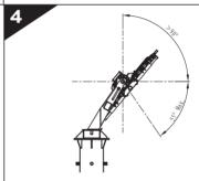
Adjust the angle of the luminaire and then tighten the handle of the luminaire's bracket.
