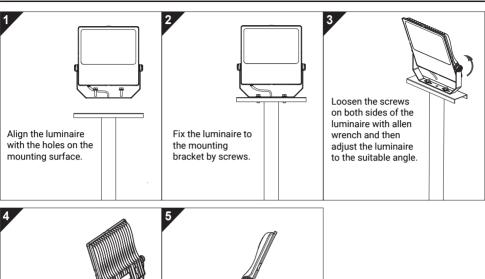
Tighten the screws on both sides of the luminaire with allen wrench and connect the wiring.
