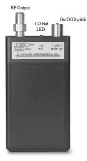
NOTE: Do not connect this noise source to a system that contains active carriers (such as TV channels, data, etc.) This noise source will cause disruption to those services.
