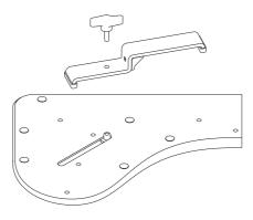
Turn the Universal Armsupport upside down on a flat surface. Loosely attach the brackets to the Armsupport by using the thumbscrew in the hole in the small arch in the bracket.
