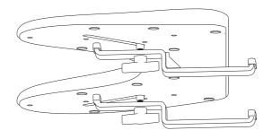
Slide your Universal Armsupport with brackets attached onto your desktop. Adjust the position as needed by sliding thumbscrews up and down the metal rail. Tighten slightly.
