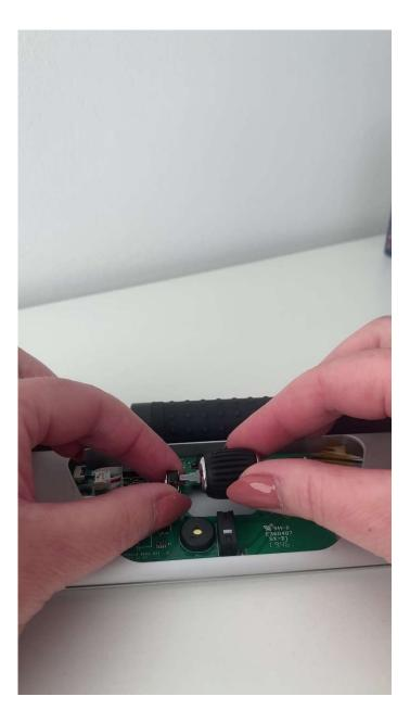
Remove the scroll wheel, by slightly pulling and lifting to the right, it will become loose of the 2 holes that holds It in place.
