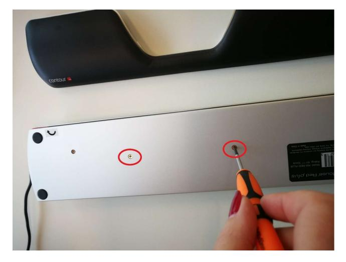
These two middle screws need to come out from the underside.
