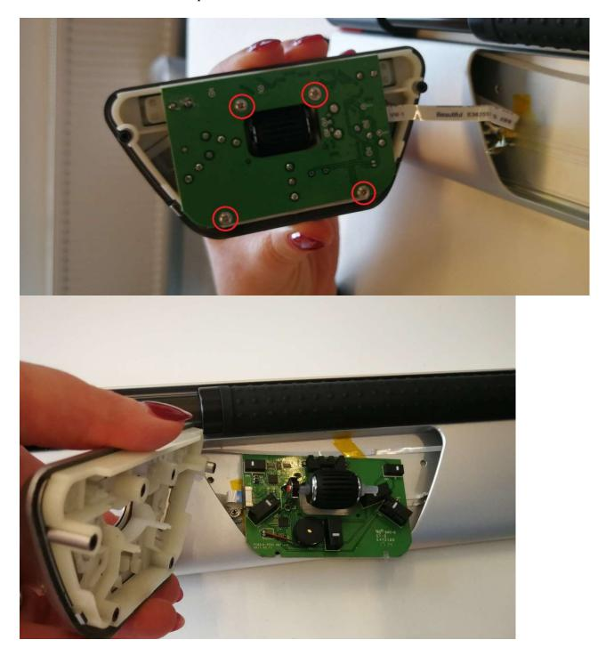
Unscrew these 4 screws to separate the board from the buttons.
