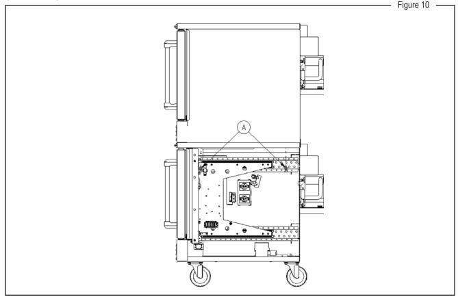
9. Replace the right side insulation, exterior panel, and lower front panel that you removed in steps 4, 5, and 6 of this procedure.
