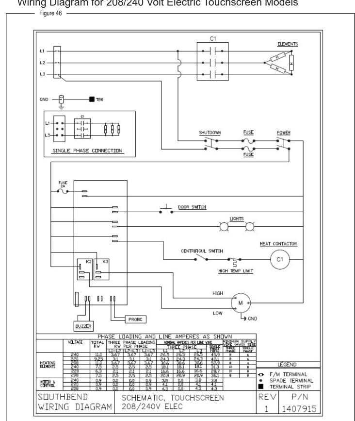
Wiring Diagram for 208/240 Volt Electric Touchscreen Models
